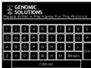
6. Enter a name for the protocol of up to eight alphanumeric characters using the alphanumeric buttons, noting the following:
