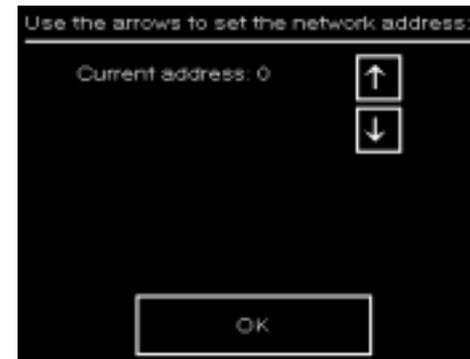
2. Use the up arrow and down arrow buttons to change the network address displayed to the left. Use "1" for the instrument closest to the controlling computer.
