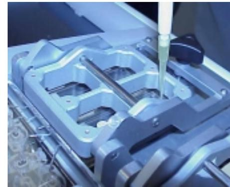
The labeled sample must fill up to the top diffusion channel. This area accommodates thermal expansion and contraction of the fluid and fluid displacement due to minor thermal expansion of the slide cover.
