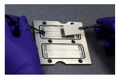
After removing the slides, be sure to rinse the HybChamber promptly with distilled water and dry
