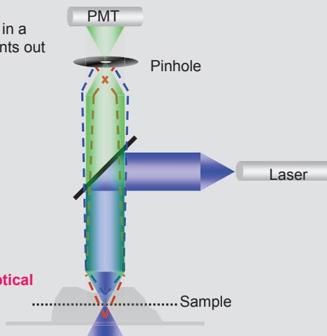
The pinhole diameter directly controls the thickness of the **optical section** .
