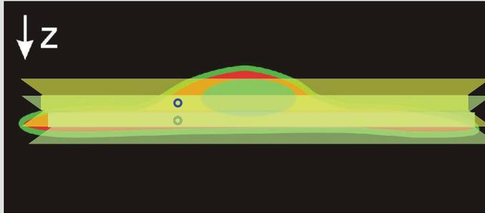
Structures which are „out-of-focus“ become visible in conventional widefield-fluorescence. Because of the focal depth inherent in all objectives, they are visible as an image blur (haze, image fog).
