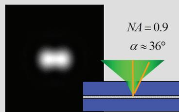
The higher the NA, the better the resolution of the microscope.
