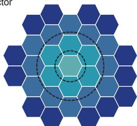
The offset of individual detectors to the optical axis provides **additional spatial information** in Airyscan (detectors of a „conventional” LSM just integrate all light passing through its pinhole).
