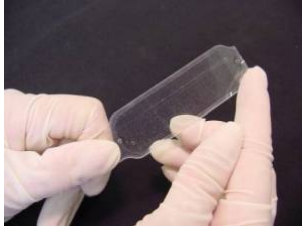
Figure 18: Release Liner Removal
